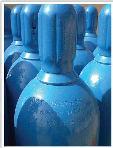
**Gas bottles and gas cylinders are usually tested using 2 techniques simultaneously: Visual inspection & Hydraulic test. These techniques are easy to handle and may be sufficient for some applications.**
